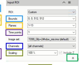
It scale the dataset reducing the size. The measurements will not be influenced by the scaling factor.
